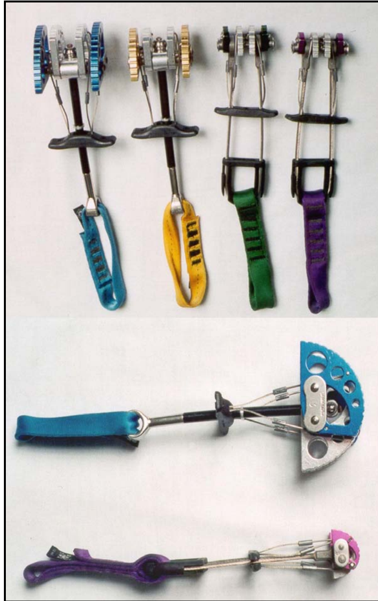
Figure 3-17. Spring-loaded camming devices.
